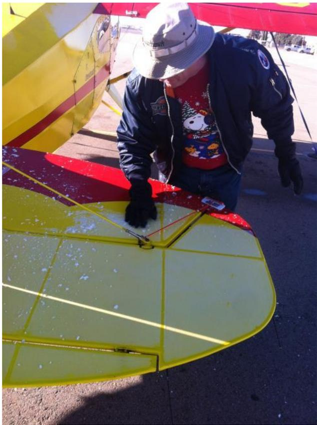
**Rubbing off frost after it melted enough to release from the surface**
