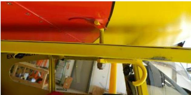
I was always a little concerned about this setup, since all of the loads were taken in bending on a fairly thin sheet of aluminum. I knew that one wrong pull on the window
