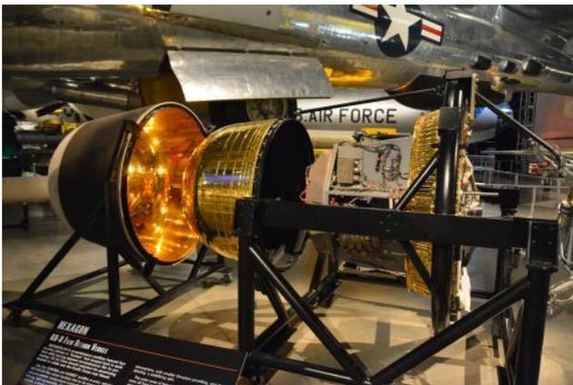
**KH-9 Film Return Vehicle, aka "bucket". This was plucked from the air under parachute by a C-119 Boxcar or C-130 Hercules. This system was made obsolete by the development of high resolution digital photography and real-time telemetry delivery of imagery**
