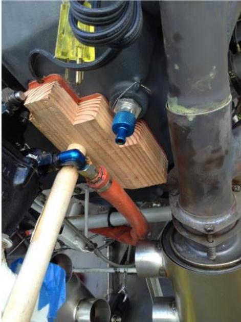
Pressure was applied to the broomstick using a small floor jack. Care was used to not apply too much force, stopping when the broomstick started to buckle.
