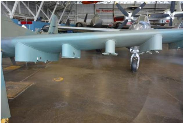
**One of the major downfalls of the design was using gravity fall bomb racks rather than ejector racks. The aircraft was fast enough to build enough aerodynamic forces that the weapons would not fall away immediately after release, causing problems with accuracy**
