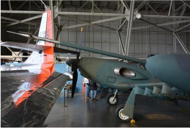
**Yaw, Angle of Attack, Pitot-Static (YAPS) boom on left wing tip tank**
