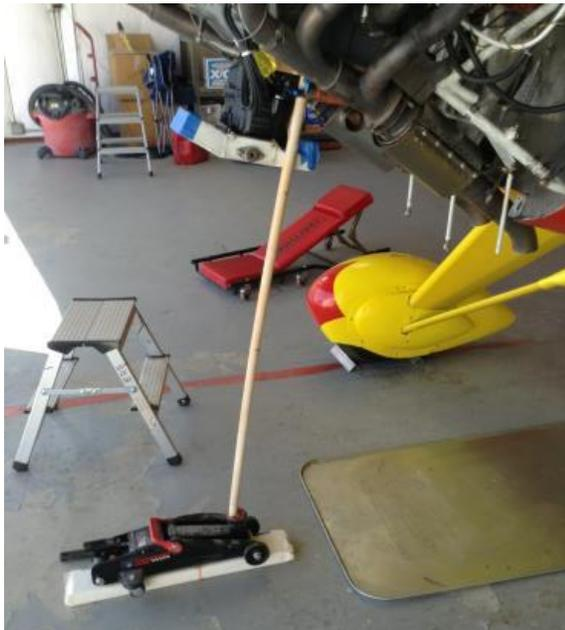
To keep the jack from rolling out of position it was placed on a 2x4 so that the wheels were off the floor. The 2x4 appears white because it was wrapped with paper from a previous use.
