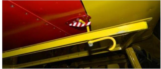
I alodined the new parts and was just going to install them that way because the effort of setting up a paint booth and priming and mixing up the two-part paint wasn't worth it for just two small parts. The **Kommandant** suggested that I should at least try to find a can of rattle-can spray paint ("Krylon") that was sort of close to the right color, acknowledging that the color match would not be perfect, but would look good enough from a distance.
