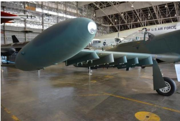
**The PA-48 was a ground attack aircraft based on the basic design of the P-51 Mustang with a turboprop engine**
