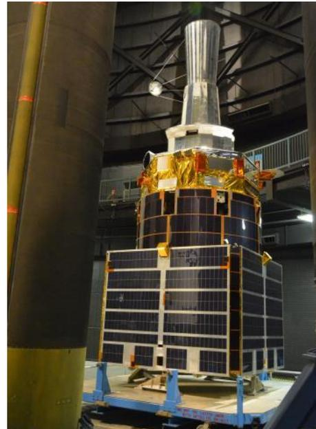
**DSP satellite structural test vehicle**
