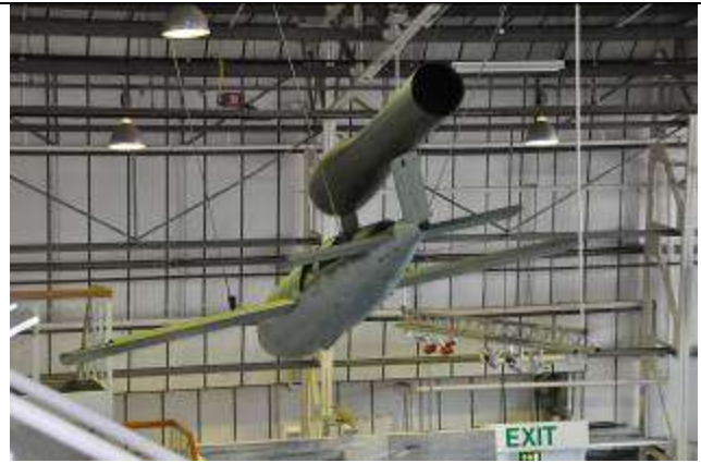
A German V-1 with its pulse-jet engine, a design that was never used on another operational design, but it still shows up in every book on jet propulsion.
