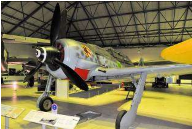
This Focke Wulf Fw190A-8/U-1 was converted from a single seat to two seats for conversion training of pilots from slower ground attack units. I wonder if RAF Museum London is interested in the USAF TPS qual eval program...
