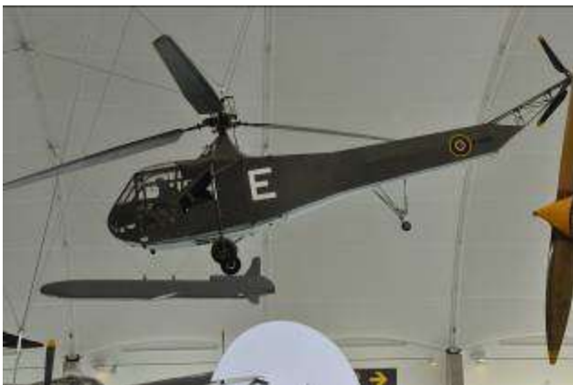
Sikorsky R-4B Hoverfly, the first operational helicopter for the USAAF and the RAF. The payload was just barely enough to carry the fuel and the pilot. Filling the second seat was almost an overload condition, sort of like the Bell Model 47.
