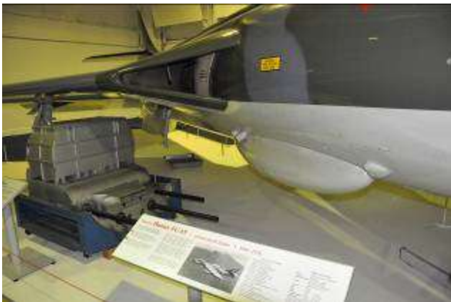
The Hawker Hunter FGA9 was a ground attack version of the Hunter fighter. Shown here is the cannon module.
