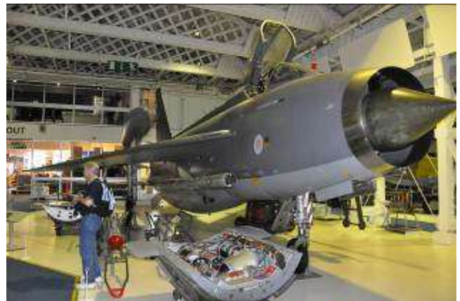
The English Electric Lightning F6 was the RAF's first supersonic aircraft. The single inlet fed two turbojets stacked vertically. After 28 years of service the type was replaced with Phantom IIs. Note that Cobra is "pushing the boundaries" himself.
