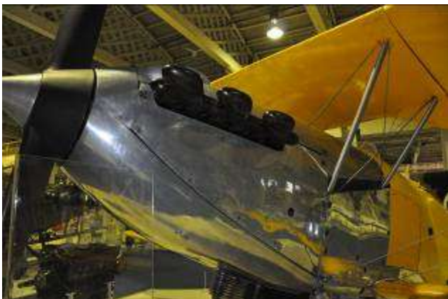
The Hawker Hart Mk II was a trainer version developed from the bomber version. This shows the Rolls-Royce FX 1B “Kestrel” engine.
