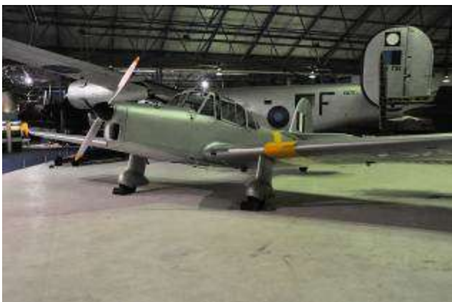
The Percival Prentice T1 was a two-seat side-by-side trainer built to replace the Tiger Moth. It was underpowered and fuel-guzzling compared to more modern American types.
