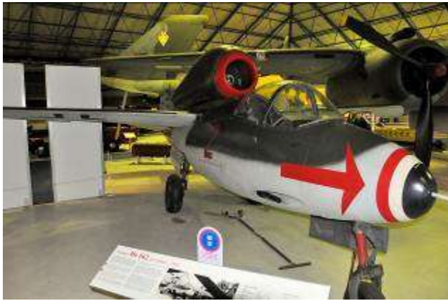
The mostly wooden Heinkel He 162A-2, another German last-ditch effort to turn the tide of the war
