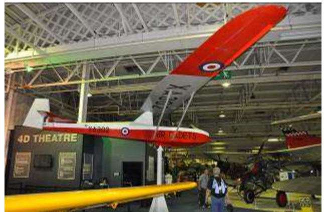
The Slingsby Cadet TX3 was a two seat training glider developed when someone decided it might be more effective than training cadets in single seat gliders.
