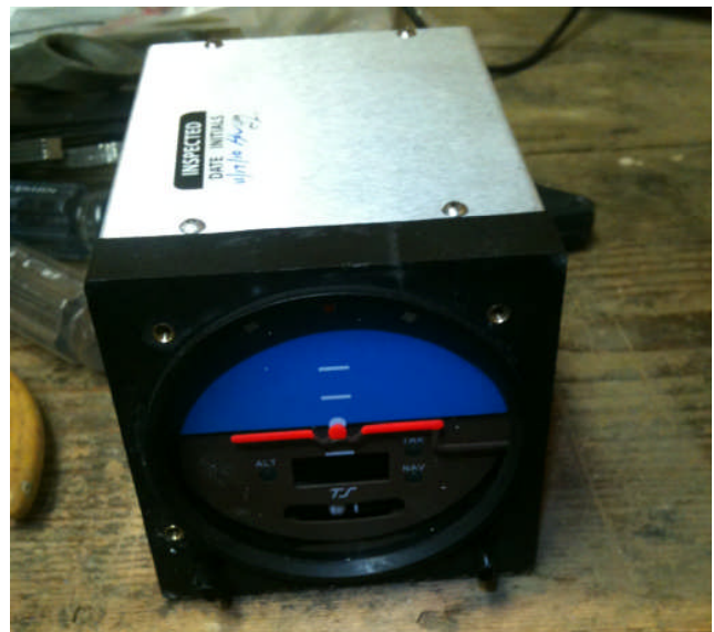
Plastic faceplate which gave an entry path for RF interference
