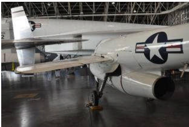
Rear view of the X-5 with the engine nozzle and showing where the main gear retracted into the aft fuselage. On the left is the side force generators of the TIFS
