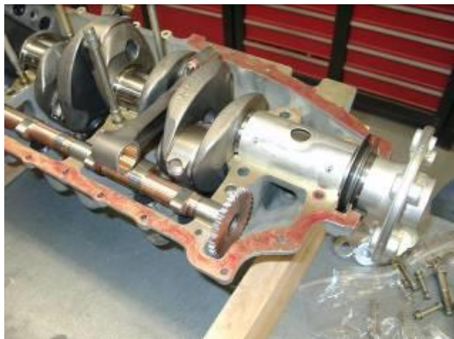
The back end of the crankcase, showing the crankshaft gear, camshaft gear, and shafts for the idler gears.
