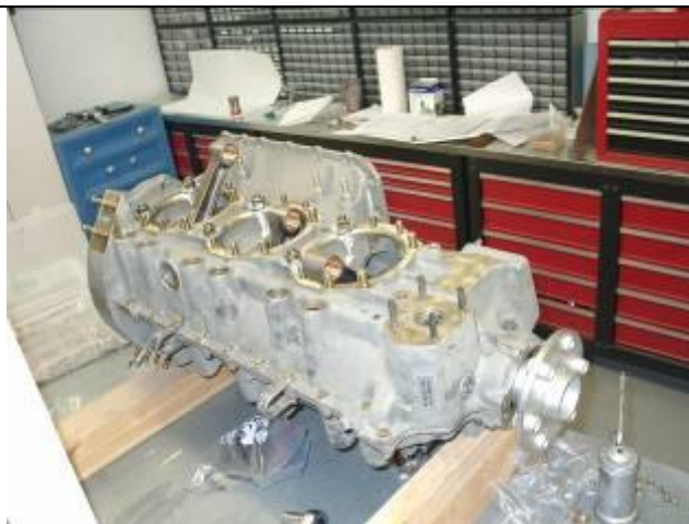
The crankcase after assembly, letting the sealant cure.
