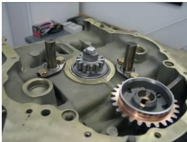
The back end of the crankcase, showing the crankshaft gear, camshaft gear, and shafts for the idler gears.
