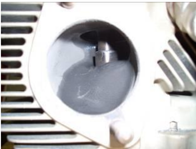
Solvent escaping cylinder head around the exhaust valve seat
