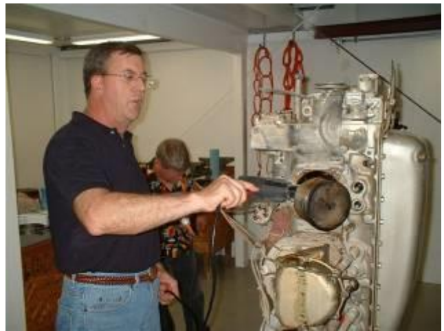
Either Bill is using a heat gun to heat the piston to free the piston pin, or...well, we can't say that in a family newsletter
