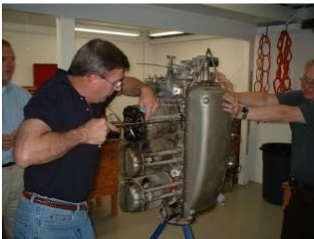
Bill removes the pushrod tube while the Kommandant tries to push him over
