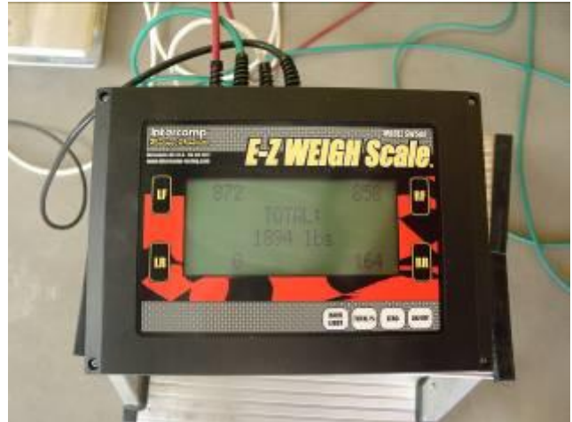
The scales in use weighing a leveled Bearhawk .
