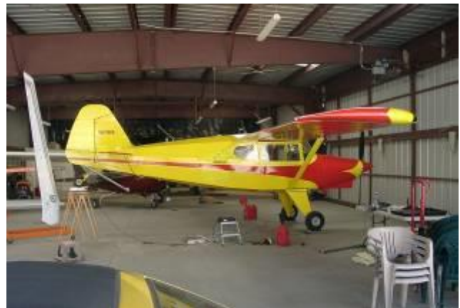
The scales in use weighing a leveled Bearhawk .
