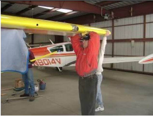
Chris Haley does his human pillar impression while Erbman rushes to get the wing root bolts in place.
