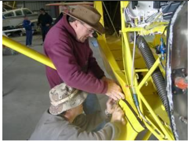
Because of very tight clearances, the nut must be screwed onto the bolt as the bolt comes up through the hole. Bill slowly turns the nut as Erbman taps the bolt farther and farther into the hole. In the background, Houdu talks to the hangar owner Jeff Pontius.
