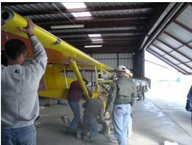
Bill and Erbman work to get the lower strut bolt in while Dave steadies the wing tip.
