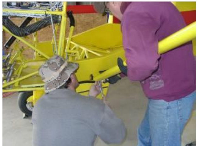
Erbman uses a tapered steel rod to line up the strut with the fuselage fitting.
