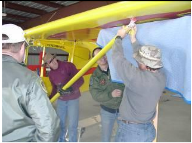
Bill holds the wing strut as Erbman lines up the top fittings.
