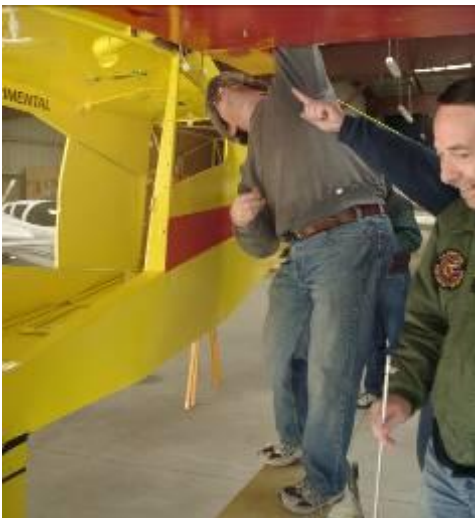
Miles points out that it's easier to put the bolts in from the top
