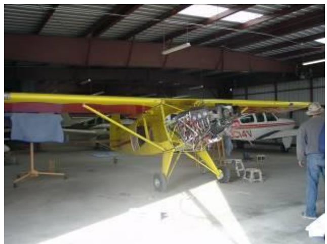
Victory! Both wings are installed with virtually no unanticipated problems.
