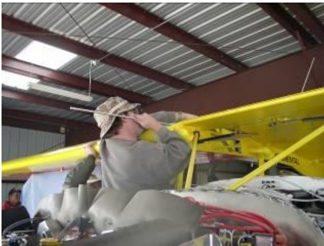
Erbman uses another tapered steel rod wiggled in the bolt holes to align the pieces prior to installing the bolt.
