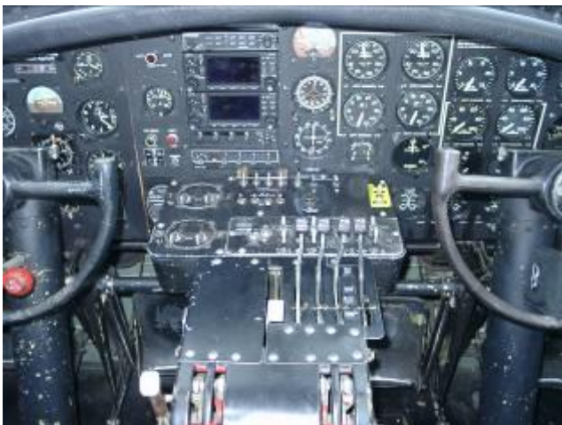
Center pedestal with mixture, magneto, boost pumps, cowl flaps, landing lights, and flap controls
