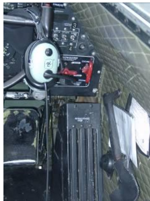
Right side of panel—engine start switches, fire extinguisher controls, and intercooler controls
