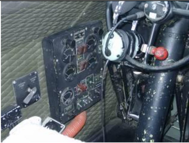
Electrical control panel on left side of pilot. Note aileron control lock (red knob) on control wheel. Sidewalls are covered in quilted fabric to cover the many wires, cables and tubes.
