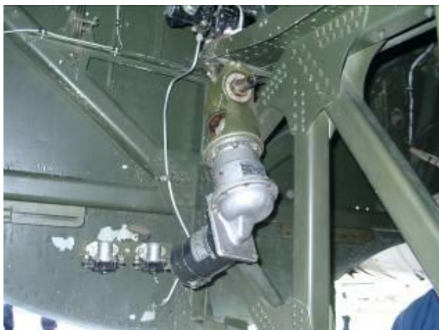
Motor for actuating the bomb bay doors, missing a few parts
