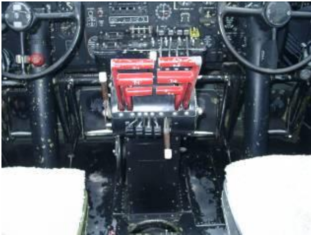
Center pedestal with red throttles and propeller controls on back (rear) end of pedestal
