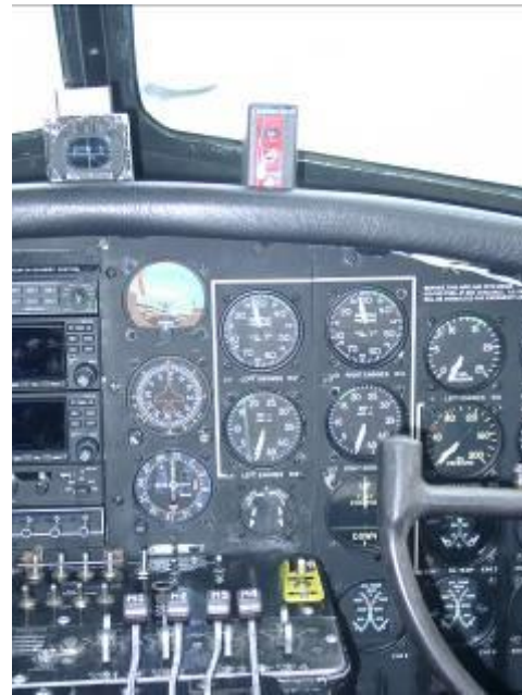
Engine instruments, with flap switch (yellow) below and landing gear switch (red) above
