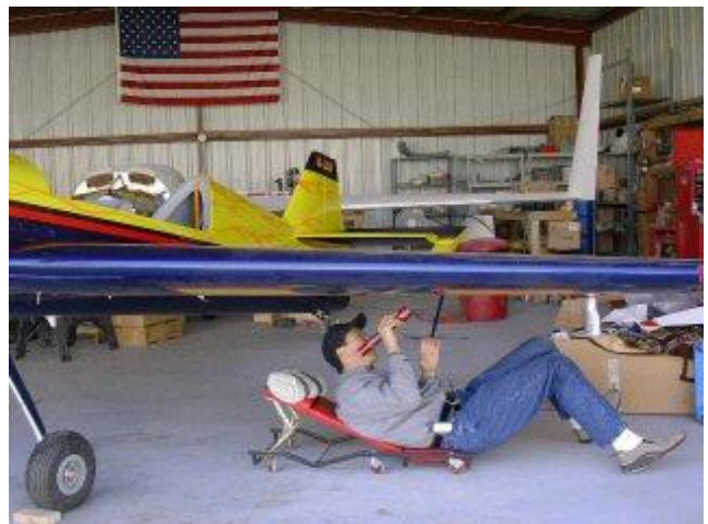
DAR inspecting the aileron attachments.
