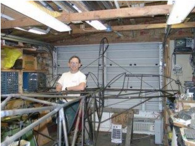
Even before the wing had left the shop, the fabrication of the fuselage began. The top was built in a jig on the table (about 18" off the floor), tacked together, and then raised above the table. The table was reworked to jig the
