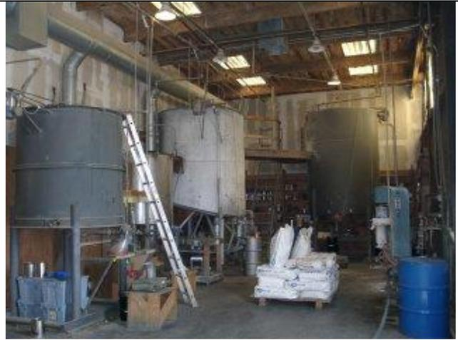
Here we see the huge vats where **Poly Brush** and **Poly Spray**, the primary coatings in the Poly Fiber process, are produced. The coatings are transferred to gallon cans using a high-tech transfer system. A highly trained and skilled Poly Fiber employee placed an empty can under a spigot at the bottom of the tank. He opened the spigot, then closed the spigot as the coatings reached the proper level. Precise measurement was accomplished using the time-honored **TLAR** system.
