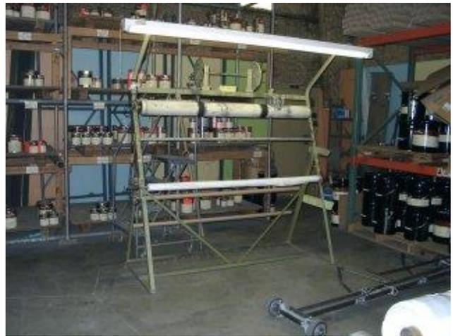
The polyester fabric arrives from the mill on large rolls, and must be re-rolled in lengths specified by the customer and stamped with the appropriate identifying mark. The fixture shown above is the actual fixture for this purpose as built by Ray Stits many years ago. This fixture is still used to this day, along with another similar fixture.
