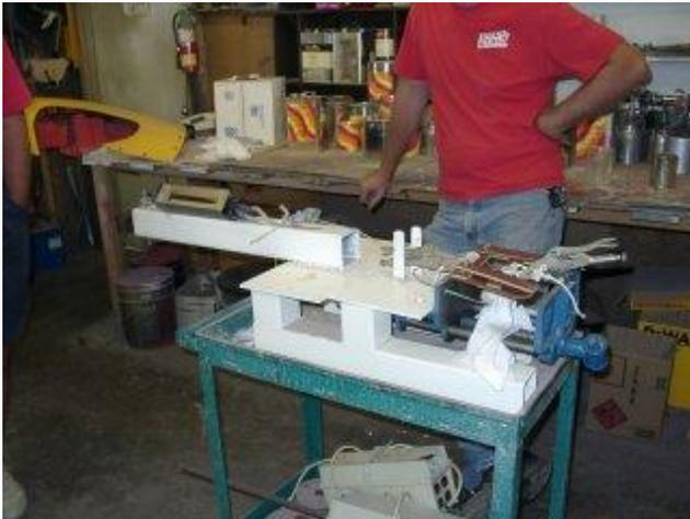
Strength and stretch of fabrics are tested on this device. The fabric is clamped into the fixture. Tension is applied by unwinding a manually powered helical inclined plane, which looked remarkably like a shop vise for woodworking. Strength is measured with a precisely calibrated spring scale.
