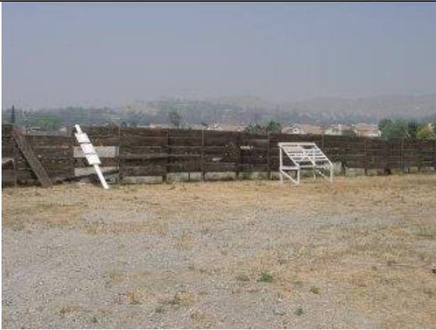
Here is a recently declassified photo of the high-tech **Poly Fiber Real-Time Solar Radiation Laboratory**. Various sample of coated and uncoated fabrics are dated and laid against this fence under the Flabobian sky to test for deterioration and fading. Additional facilities are available for accelerated testing, where samples are placed under high-intensity ultraviolet lamps for weeks instead of years to test the coatings.
