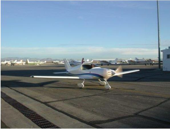
Discussions Wednesday with Chapter 49 members pointed to the cold temperatures (dense air) were causing the 2-stroke engine to run lean, so the carburetor jetting should be enriched. Additionally, the prop needs to be adjusted for some more pitch to bring the full throttle RPM back down.
